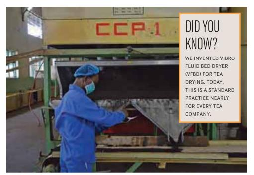
To stop the process of fermentation and to displace moisture, the fermented 'maal' is fed into driers in a regular manner; and is subjected to temperatures ranging between 121°C and 127°C, with controlled throughput time of 22 minutes to 25 minutes.
