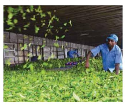
The plucked leaves arrive at our factories and are spread evenly in the withering troughs. We have large enclosed troughs where the leaves are spread evenly. We use fans that blow hot and cold air through leaves, reducing the moisture content by 28-32% (chemical wither) through a 14-to-16-hour process. We can control the air, based on the thickness of the leaves.
