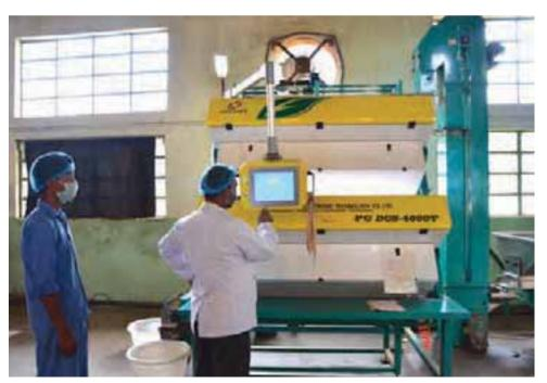
After drying, the tea is sorted into various grades and sizes by an automatic sorting machine. The Trinick Sorter was invented and patented by John Trinick, one of the pioneers in tea manufacturing; he was also our advisor. This machine sorts tea with least damage and wastage.
