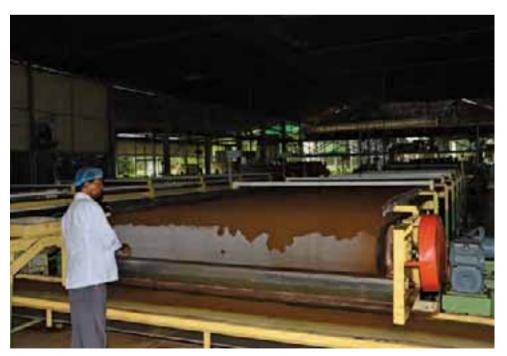
This is the oxidation process for both the CTC and Orthodox 'maal'; and lasts between 70 and 180 minutes, depending on the colour and aroma of the fermented leaf. This is the process of exposing the tea leaves to atmospheric oxygen under controlled conditions of humidity and light.
